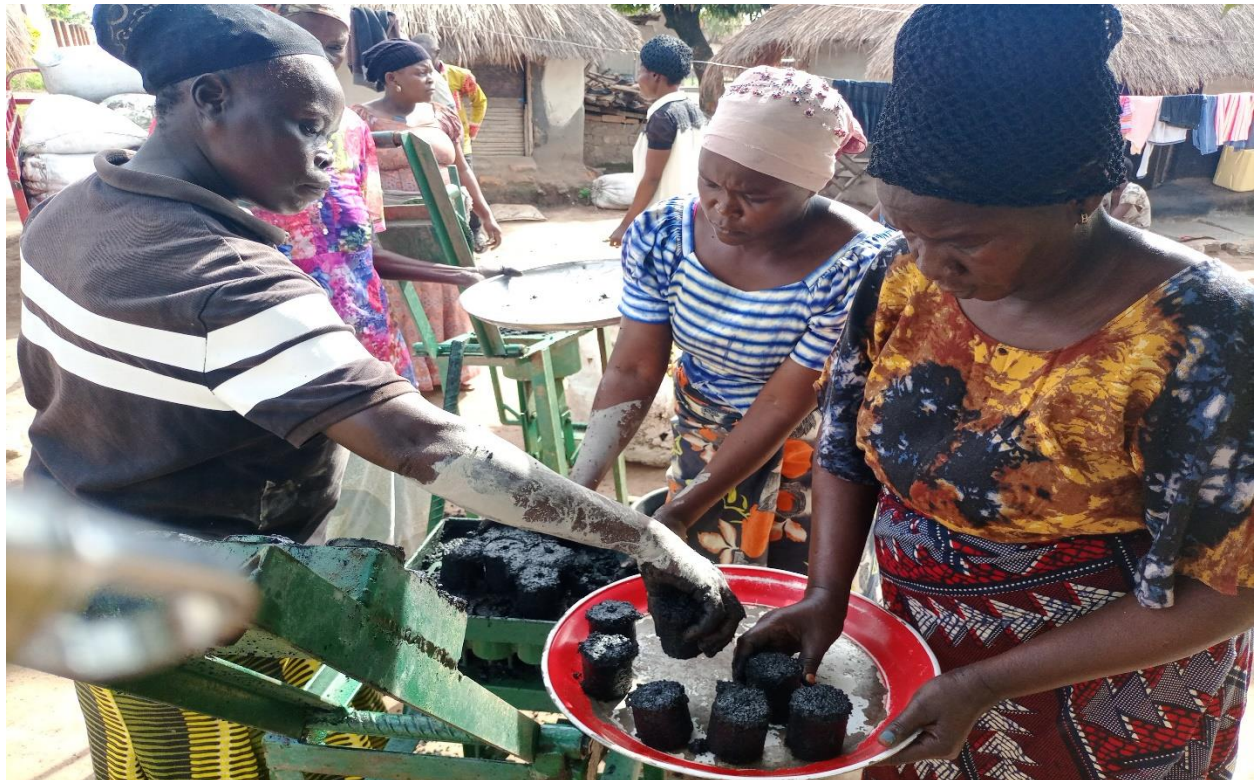
Giant Role Model group members removing briquettes for the small stove from the machine and arranging them on a tray ready to be taken into their store.
